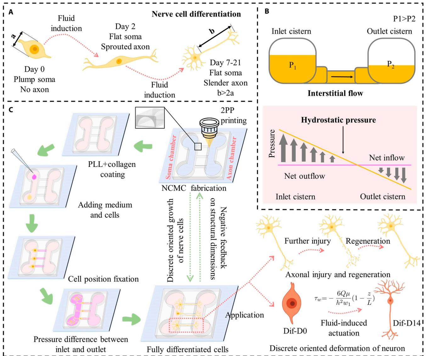
**Fig. 1.** Schematic of the two-photon polymerization (TPP)-based method for optimizing the nerve cell growth in the microchannels of nerve cell culture microfluidic device (NMC). (A) Differentiation process of nerve cells. (B) Interstitial flow caused by hydrostatic pressure drives the deformation of differentiable cells. (C) Overview of the TPP-based method for optimizing the nerve cell growth in the NMC microchannels and its application.
