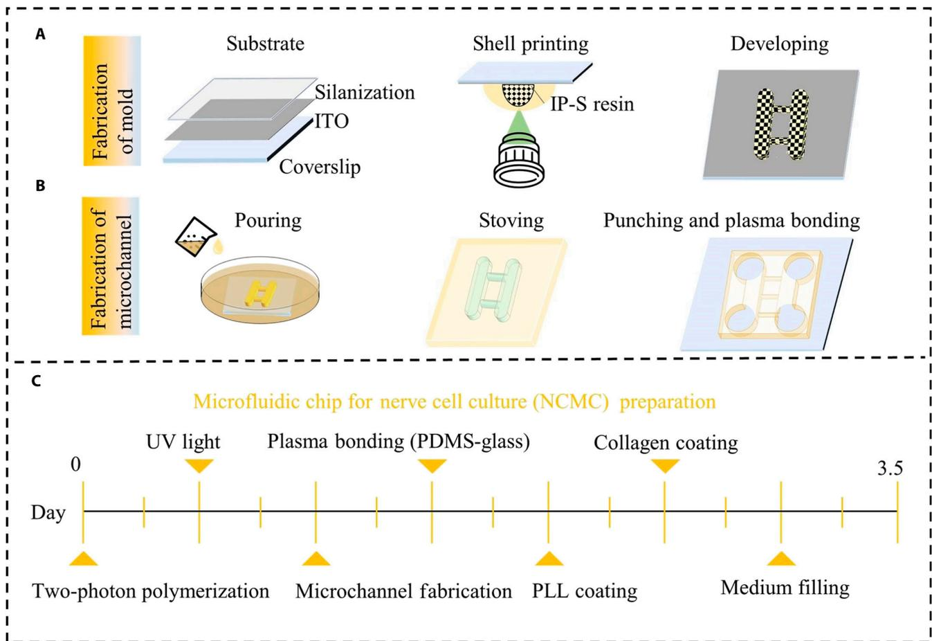
**Fig. 2.** Fabrication processes of the NCMC. (A) Fabrication steps of the NCMC mold based on TPP printing. (B) Fabrication steps of the NCMC based on the NCMC mold. (C) Specific timeline for the NCMC preparation.
