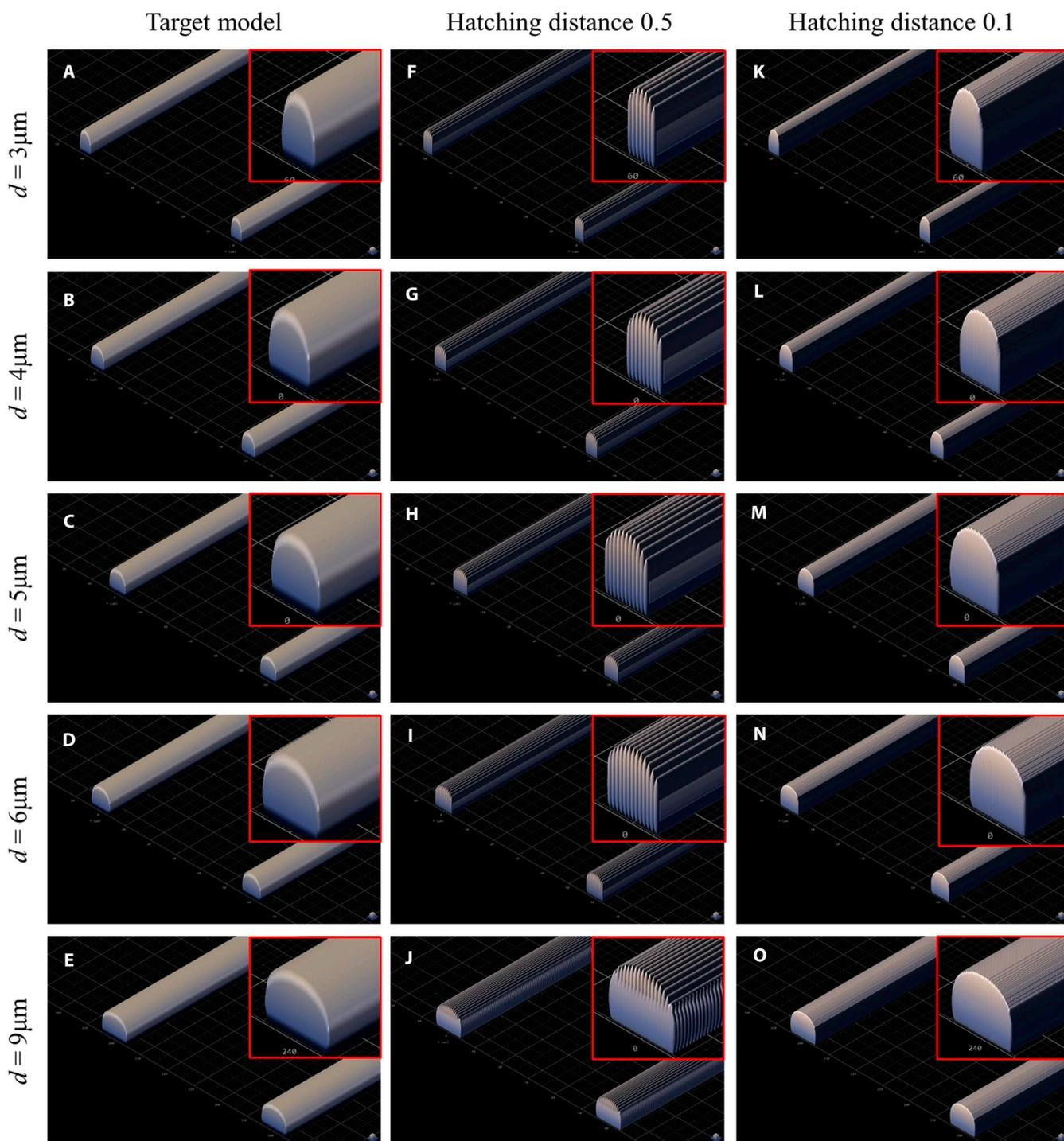
**Fig. 3.** The Describe model based on TPP printing for molding the microfluidic chip with 3D micro-topography (upper right-side view). (A to E) Molds with microchannel width are 3, 4, 5, 6, and 9 respectively. (A) to (E), (F) to (J), and (K) to (O) respectively represent the Target model preview, the model preview with hatching distance (printing resolution) of 0.5, and the model preview with hatching distance of 0.1.
